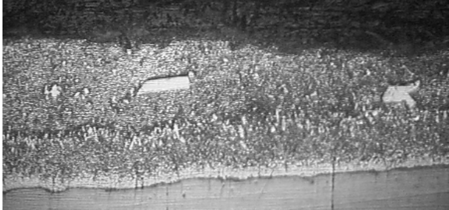
Pic 3 – HDG Double dip process. Coating consists of multiple layers of different Zn-Fe alloys. White areas in the outer coating are Zn-Al alloy particles
